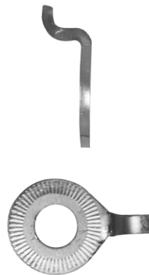
Special safety washer - must be mounted on all bikes with disc brakes, unless the fork has reversed fork ends
