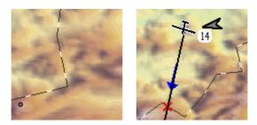
The final glide path is checked for whether the glider clears terrain by the terrain clearance height. If clearance is not attained, a red cross appears on the map at the point where the violation occurs. No icon is drawn if there is no task defined.
