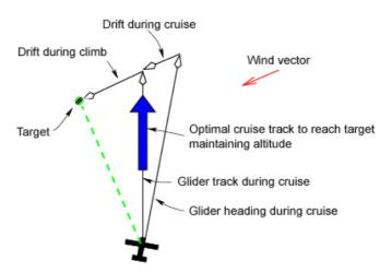
The optimal cruise track is displayed on the map area as a large blue arrow, and it recommends the glider steers so that the glider's track is lined up with the blue arrow during cruise such that it will arrive at the waypoint in minimum time. When the wind is negligible, or when the computer is in final glide mode, this arrow will point along the black line that indicates the track to the next waypoint.
