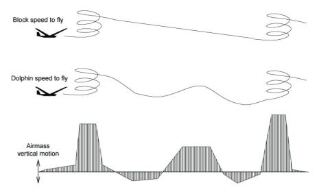
A configuration option 'Block speed to fly' (see 11.5) can be used to specify whether dolphin or block speed to fly is used. The InfoBox 'V Opt' shows the optimum speed according to whichever mode is selected. When connected to the Vega intelligent variometer, the speed command sounds are based on this optimum speed value.
