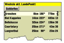
This dialog contains a list of maximum ten landing points. For each landing point, type (A: Airfield, L: Landable field), distance, course and altitude difference to safety altitude are displayed as well as the required glide rate to reach this point. The list is sorted by glide rate and landing point type (airfields are at the top). Red highlighted list elements are landing points which are near but not reachable according to the computers calculations.
