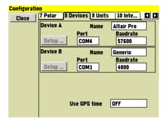
Two COM devices are available (device A and device B), to allow, for example, one to be connected to a GPS and another to be connected to a second device such as a variometer. If there is no second device, set the device B port settings to the same as those of device A – this instructs the program to ignore device B.
