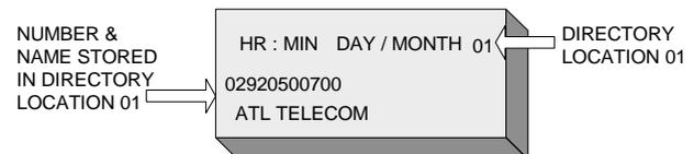
Either, use the UP (▲) or DOWN (▼) key to scroll through the Directory entries until the required entry is displayed or use the keypad to locate the relevant area of the directory. E.g. pressing the "2" key three times will bring up the first entry beginning with "C" etc.
