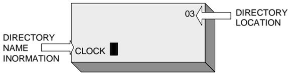
Edit the Name using the keypad (e.g. two presses of the "2" key will produce a "B"). Press the LEFT (◀) or RIGHT (▶) key to move to the left or right respectively. Press and hold the (◀) key to delete the current character. Press and hold the (▶) key to delete all characters on the display. Use the STAR "\*" key to move the cursor to the left. Use the HASH (#) key to move the cursor to the right. Use the ZERO (0) key to enter a space.
