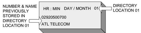
Either scroll through the directory using the UP (▲) or DOWN (▼) key for the required number, or use the keypad to search the directory for a stored name, e.g. pressing key "5" once will bring up the first name stored, beginning with the letter "J".
