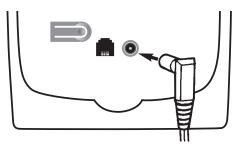
2 Plug the power supply unit into the wall socket
