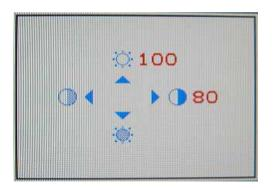
When user press the **Up** or **Down** keys under none OSD status will trigger this menu appear for Brightness and Contrast adjust. This menu will display about 20 seconds.
