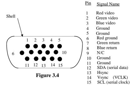
Signal cable input connector.
