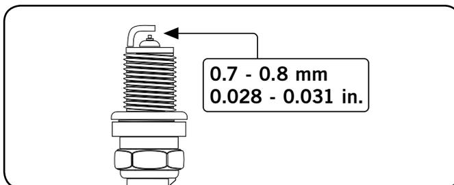
5. Refer to the spark plug recommendation chart when replacing the plug.
