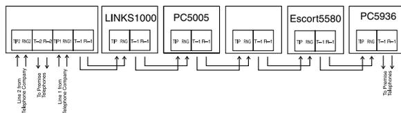
For example, if you are installing a PC5005 with a LINKS1000/GSM1000 and a PC5936 Intercom module, connect the incoming line to the LINKS1000, then from the LINKS1000 to the PC5005, then from the PC5005 to the PC5936 Intercom and then from the PC5936 to the house telephones.
