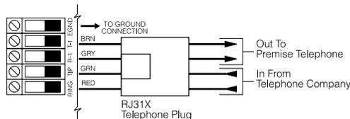
Connect the PC5005 and modules that use the telephone line(s) in the following order:
