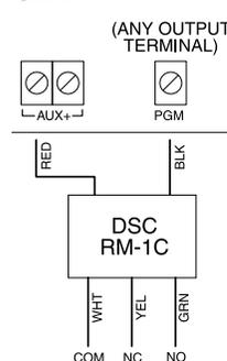
Each PGM output is designed so that when activated by the panel, the terminal will switch to ground
