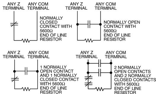
End of Line Resistors . . . . . Section [013], Option [1]
