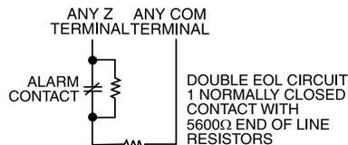
**NOTE:** If the Double EOL supervision option is enabled, all hardwired zones must be wired for Double EOL resistors, except for fire and 24-hr Supervisory zones.
