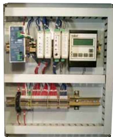
Interface Panel without Enclosure
