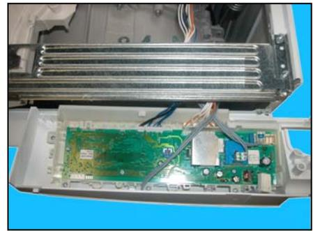
b. Remove the screws and release the hooks which secure the board casing to the control panel.
