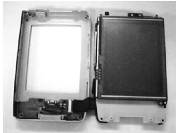
5. After removing FPC from the connector assembled onto the upper case assembly, remove the upper case assembly as shown to the right photograph.
