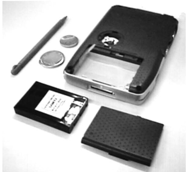
2. After peeling item 54 PLATE, be sure to remove a screw assembled behind this plate as shown to the illustration and below photograph. Otherwise, the lower case (the upper case) assembly can not be removed as described in **EXPLODED VIEW** in this manual.
