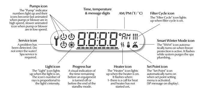
2- heater has just turned off and element is cooling down or 3 - not enough current available to start heater
