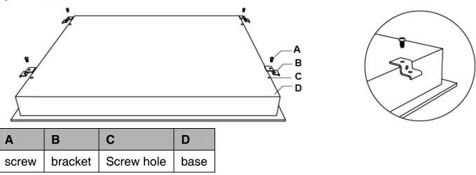
Adjust the bracket position to suit for different work surface's thickness.
