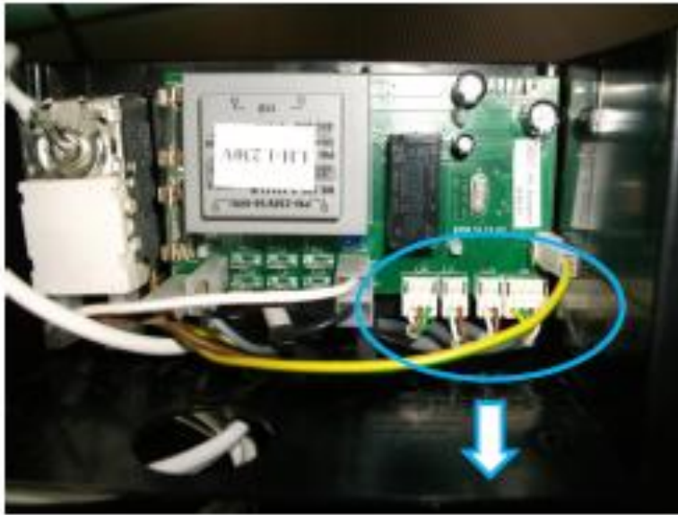
7. Disconnect the sensor sockets from the electronic card
