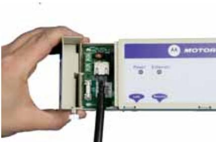
**Step 4:** Put the cover back and tighten the screw.
