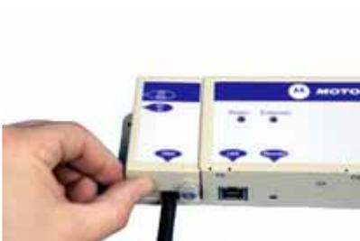
**Step 5:** Plug in power lead using a cable appropriate for the installation.
