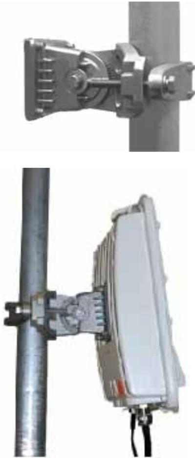
**Step 3:** Adjust the elevation and azimuth of the unit before tightening to the required torque settings of 14 Nm (11 lbft) for both bolts.
