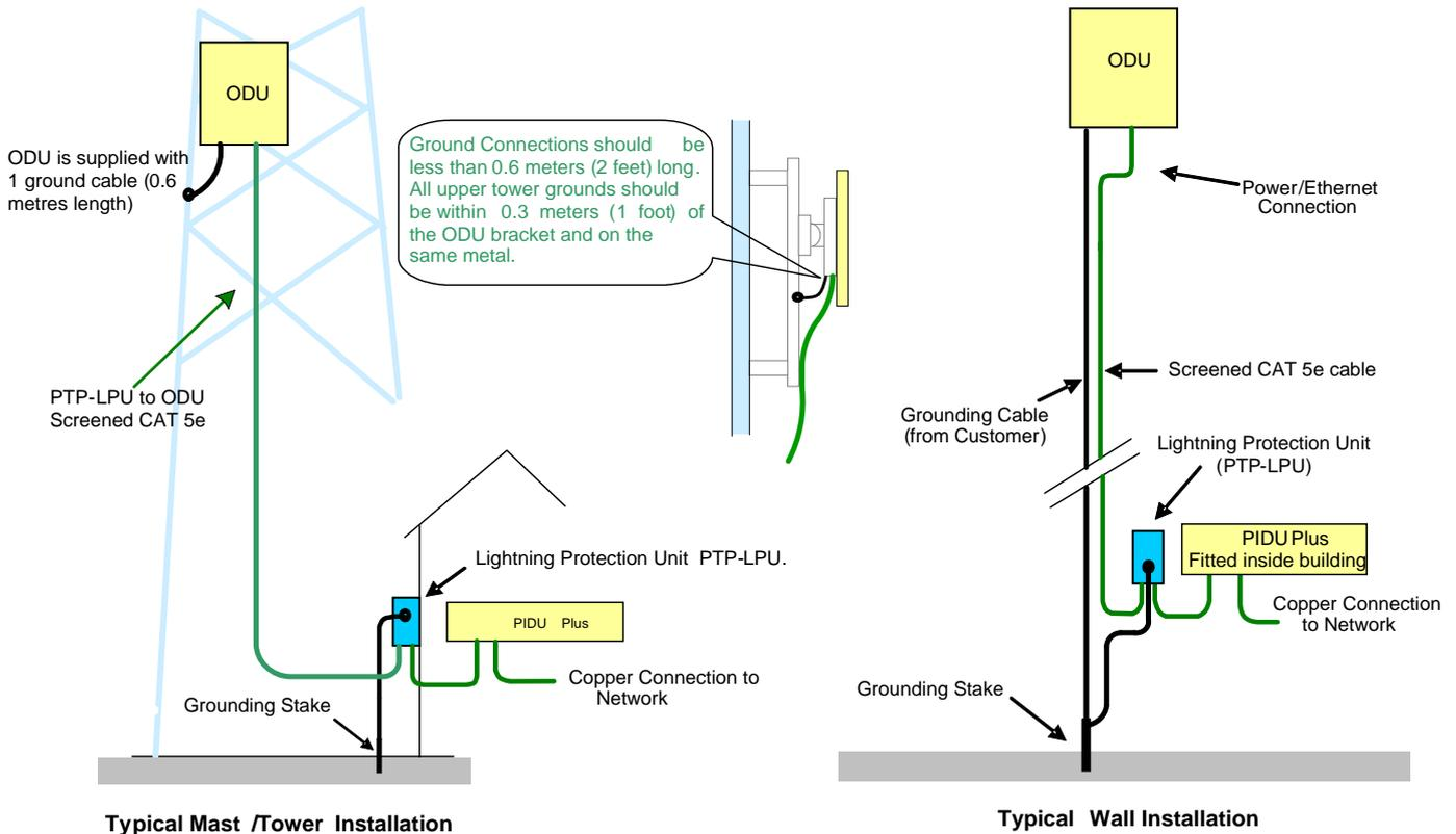
The recommended standard components for protecting installations are:
