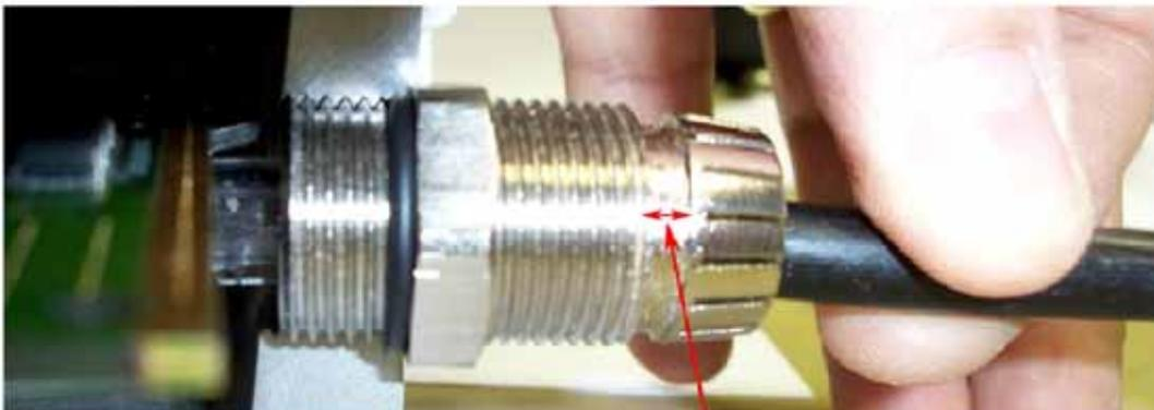
**Apply small movements to the cable until you see a gap here before unscrewing the gland body.**
