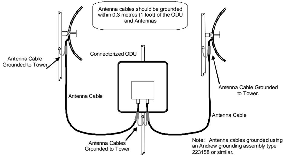
Additional Grounding Requirements for Connectorized ODU
