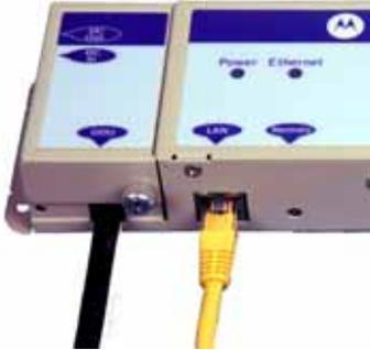
**Step 7:** 30 seconds after powering, the Ethernet LED should be observed to flash slowly 10 times. If the Ethernet LED does not illuminate (orange), then either the PIDU Plus or the cable to the ODU may be faulty. Replace cable and/or PIDU Plus and repeat from Step 1.
