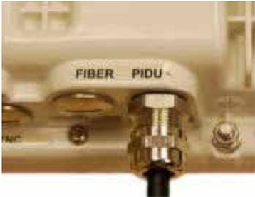
**Step 2:** Undo the retaining screw of the PIDU Plus and hinge back the cover.
