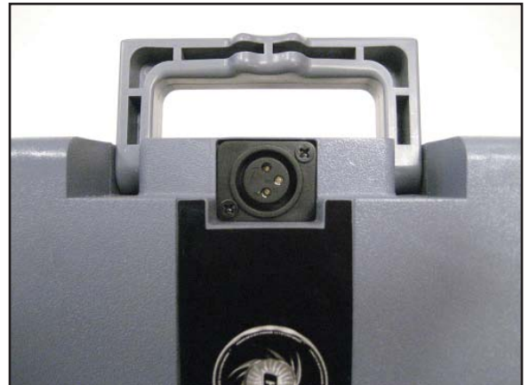
Electric Bikes with Rack Mounted Battery (RMB) Packs - Lift the battery pack handle to expose the charger port and attach charger.
