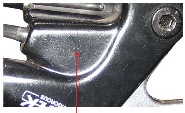
Location of microswitch housed inside of the brake lever body
