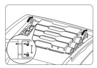
4 Remove the empty toner cartridge. Place the used cartridge in a plastic bag to avoid toner spillage and discard the empty cartridge.
