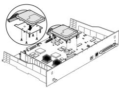
Fasten the hard disk to the bracket with the screws provided.
