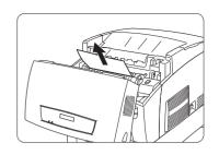
4 Push both fuser unit levers completely back.
