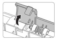
3 Lift the clip at the end of the media feed rollers ①, and remove the media feed rollers ②.
