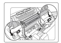
4 Lock the transfer cartridge into the printer by pushing down on the base of the tabs until you hear a click.
