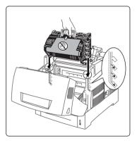
9 Remove the black protective sheet and dispose of it.
