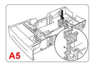
**d** To return to other approved media sizes, remove the A5 spacer from the slot, and then replace it in the tray.
