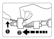
4 Align the new media feed rollers' axis with the shaft in the media tray as illustrated and slide the shaft through the roller until the clip locks into the groove at the end of the shaft.
