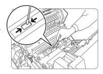
Replace the transfer roller by inserting the pins at both ends of the transfer roller into the U-shaped bearings inside the printer.
