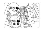
6 Lift up both levers of the fuser unit.
