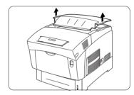
3 Gently rotate the toner levers to the unlocked (backward) position.
