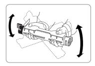
7 Align the toner cartridge with the cartridge guides. Gently push the cartridge into the printer.
