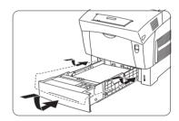
Check the gauge to make sure the tray is registering the loaded media. Use this gauge to determine when the tray needs to be refilled.
