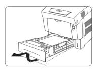
2 Hold the tray with both hands, lifting slightly, and remove it from the printer.
