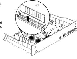
6 Insert the new DIMM straight down into the DIMM connector until the latches snap into the locked position.
