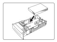
■ Multipurpose Tray—Open the multipurpose tray, adjust the media guides to the width of the transparencies, and then place the transparencies into the tray with the printing side up.
