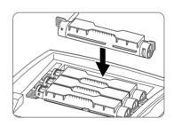
8 Gently rotate the the toner levers to the locked (forward) position.
