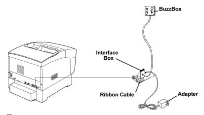
The BuzzBox's ribbon cable is designed to be directly attached to the printer's parallel port, not to an adapter or an additional cable.
