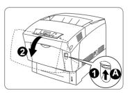
**3** Grasp the two tabs ① on the transfer roller to lift it straight up ② out of the printer.
