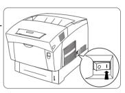
After approximately 6 minutes warmup (assuming normal temperature and humidity), your printer prints a startup page and displays "IDLE" on the message window.
