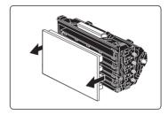
8 Gently guide the imaging unit straight into the printer, following the arrows on the printer to seat the pins.
