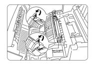
7 Grip the unit's levers, and gently lift it out of the printer.
