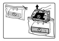
6 Holding the imaging unit horizontally, carefully pull the tabs straight out and completely away from the unit.
