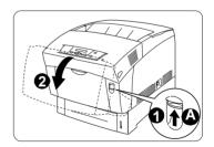
2 Remove the jammed media. Remove any torn pieces of paper still in the printer.
