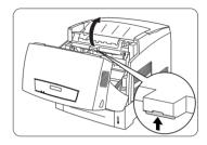
4 Remove the used imaging unit.
