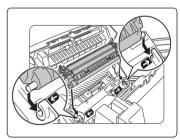
6 Push down on the two tabs until they click to lock the transfer roller cartridge into the printer.
