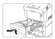
12Remove the media tray cover from the rear of the printer.
