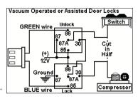
the voltmeter will receive "+12 volts". Cut this wire and make your connections. Be sure to program the door lock timer for 3.5 seconds.
