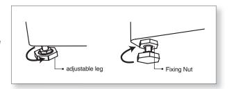
3 Make it sure that the washer does not sway when you press down the four corners of the washer's top plate.
