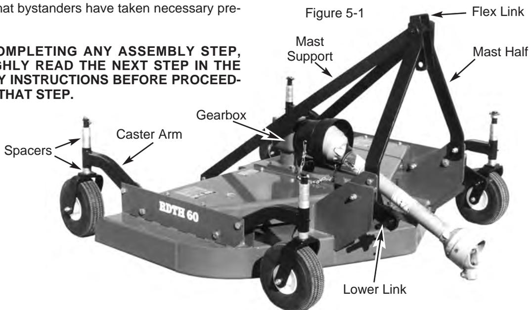
E. Fasten mast supports and upper flex link to mast halves using 1/2 x 5" bolt, pivot tube and locknut.
