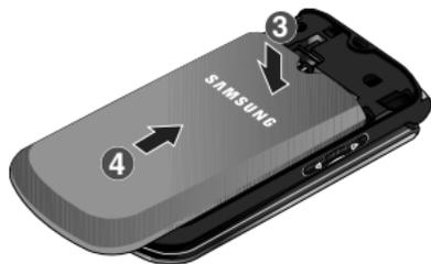
4. Press lightly on the bottom end of the battery up over the battery until it clicks into place.
