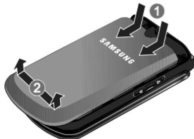
3. Lift the battery up (1) and away (2) from the phone, bottom end first.
