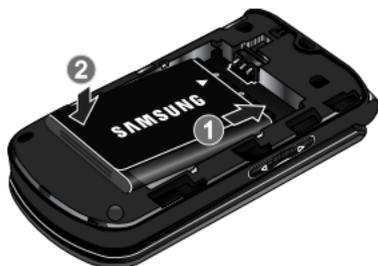
2. Press lightly on the bottom end of the battery down into the phone until it slips into place.
