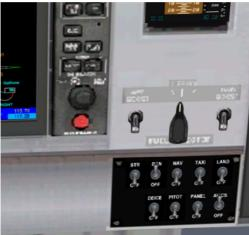
Then look on the rightside at the switches. The bottom row, first and second from the left are for deicing and pitot heater.
