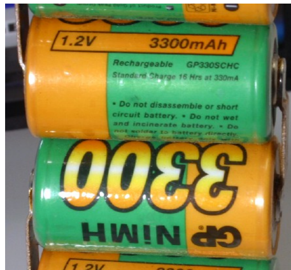
Figure 8. Close up of 3300 mAHr cells.
