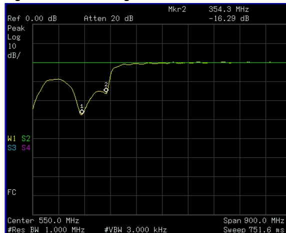
Figure 24 Measuring the Return Loss of the Filter
