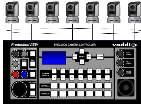
Figure 6: Two Precision Camera Controllers set up in Link Mode. The Precision Camera Controller with the cameras connected is the Primary, and the Precision Camera Controller without cameras is the Secondary unit.
