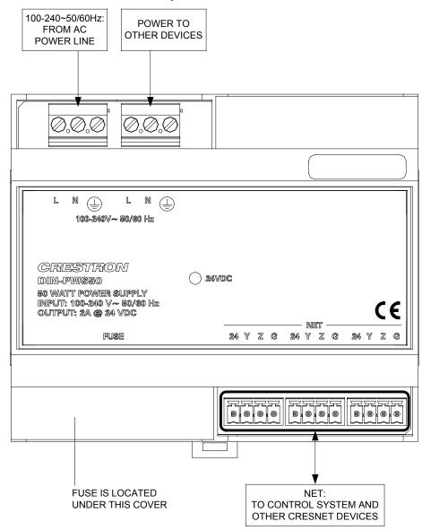
Fuse Replacement If the DIN-PWS50 does not power up when it is plugged into an AC outlet, the fuse may need to be replaced. The fuse holder is located on the front panel, under the cover in the lower left corner. To replace the fuse:
