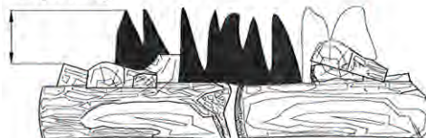
Figure 18 - Incorrect Flame Pattern with Control Knob Set to High (5)
