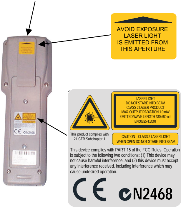
Figure 1 - F734-E Laser Safety Labels
