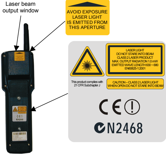
Figure 2 - F734-E/RF Laser Safety Labels
