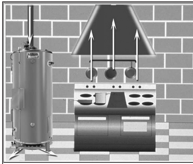
Downdraft Caused by Kitchen Vent Hood
