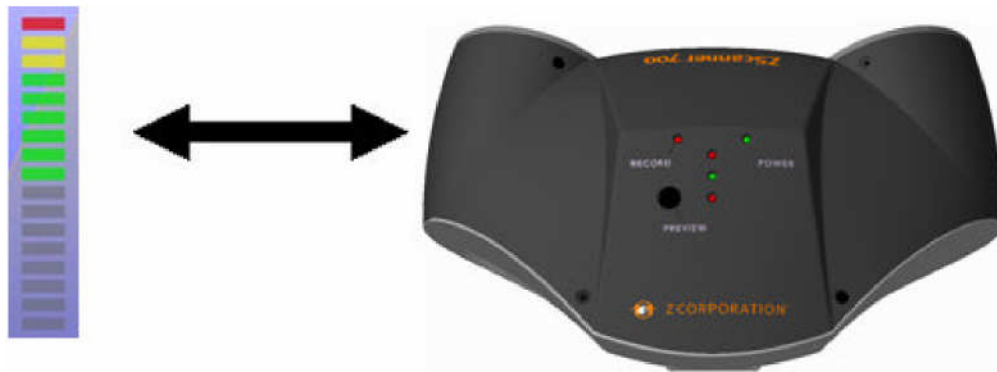
Figure 3.6 - Graphic and physical representation of the scanner too close to the surface
