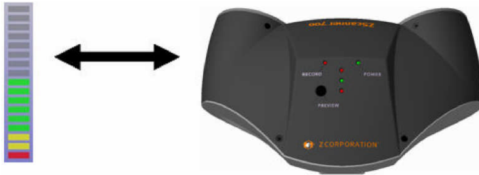
Figure 3.8 - Graphic and physical representation of the scanner too far from the surface
