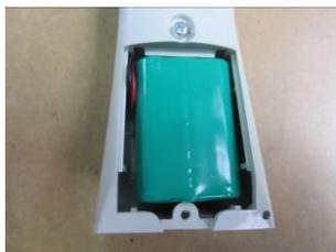
**3 Insert the battery and place the wire in the box**
