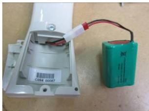
**2 Connect the battery to the connector**
