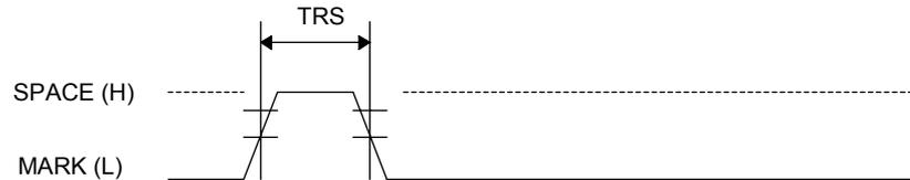
**Figure 2.1.2 Minimum Reset Pulse Width (pin 25)**
