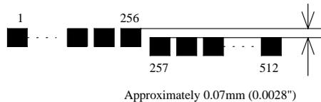
**Figure 1.6.3 Shifting of the Print Position**
