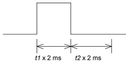
**Figure 2.2.3 Drawer Kick-out Drive Signal Output Waveform**
