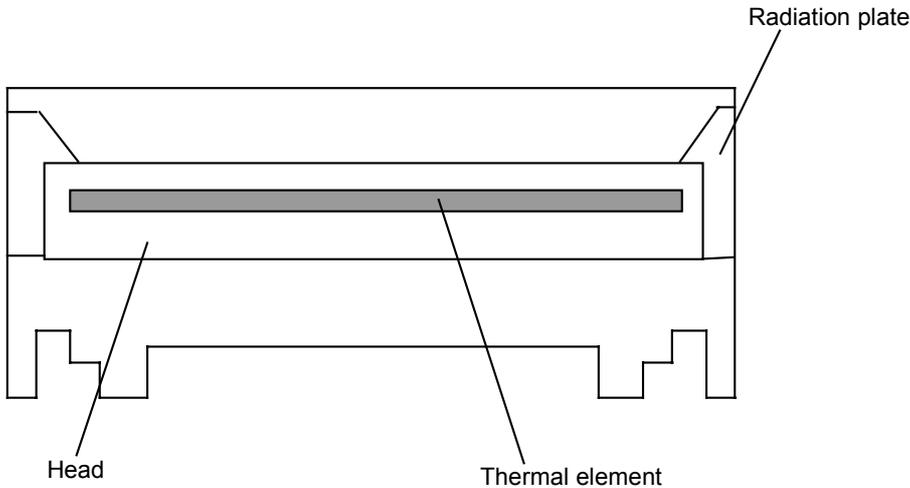
**Figure E.1 Print Head Thermal Elements**
