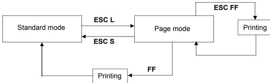
**Figure 3.12.1 Shifting Between Standard Mode and Page Mode**
