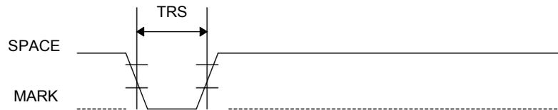
**Figure 2.1.1 Minimum Reset Pulse Width (pin 6)**
