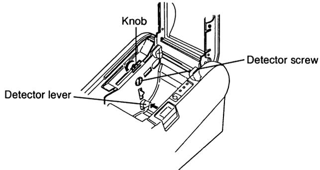
**Figure C.2 Changing the Near-end Adjusting Position**
