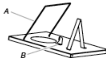
A. LP gas fuel tank retention bar B. LP Gas fuel tank holder
