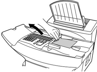
② If the leading edge of the document is protruding from the printer compartment outlet, try pulling it out.
