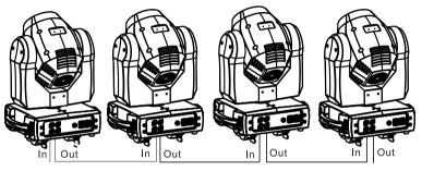
The number of daisy-chained fixtures is limited by the number of DMX channels required by the fixtures in relation to the maximum 512 channels available in one DMX universe. Note that if independent control of a fixture is required, it must have its own DMX channels. Fixtures that are required to behave identically can share the same DMX address and channels. To add more fixtures or groups of fixtures when the above limit is reached, add a DMX universe and another daisy-chained link.
