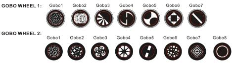
Any gobo can be projected statically, or the wheels can be rotated, both clockwise and counter-clockwise. Individual gobos on wheel 1 can be rotated both clockwise and counter-clockwise, and a gobo shake function is available. The fixture can be set to automatically blackout during gobo changes.
