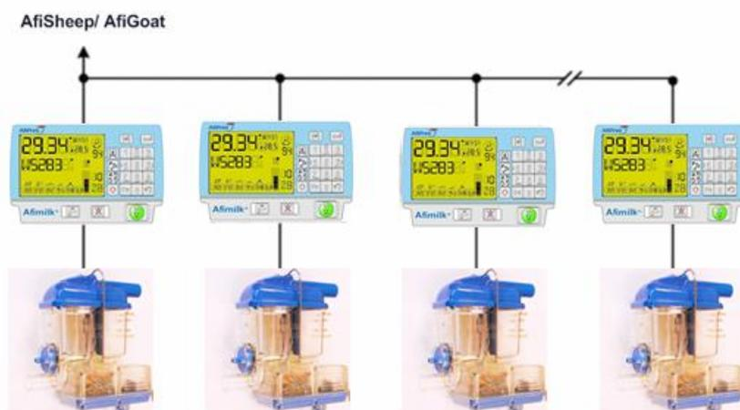
**Figure 1: Terminal 155i units connected to AfiSheep/ AfiGoat**
