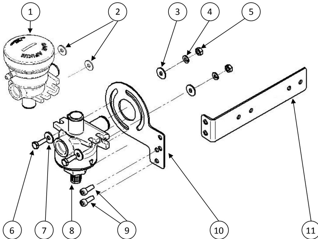
Figure 42: Parts for Attaching Vacuum Shut-Off Valve
