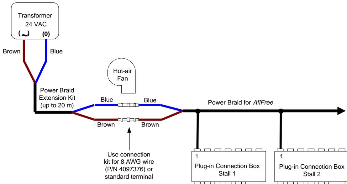
Figure 22: Power Cable Wiring
