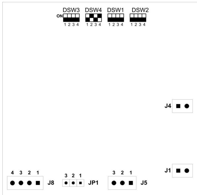
**Figure 29: Socket and DIP Switch Locations**
