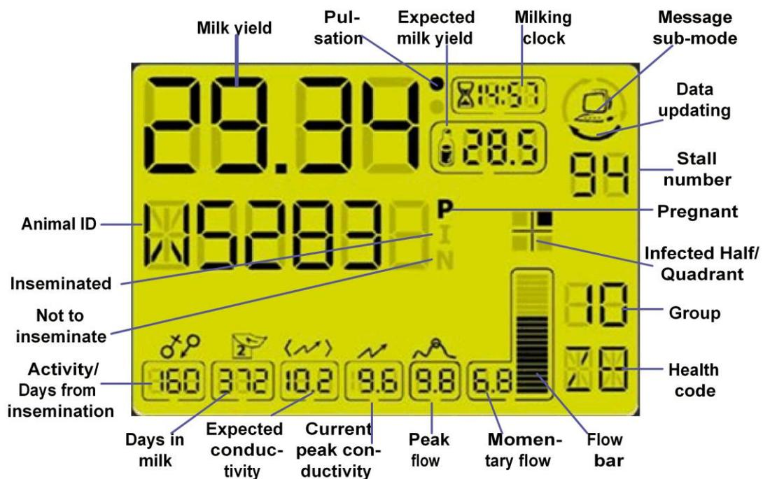
Figure 6: Terminal 155i LCD Display
