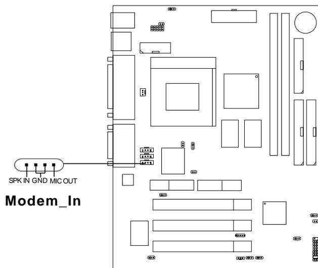
SPK\_IN is connected to the Modem Speaker Out connector.
