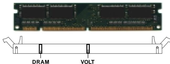
3. The plastic clip at the side of the DIMM slot will automatically close.
