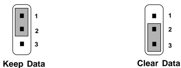
**Note:** You can clear CMOS by shorting 2-3 pin, while the system is off. Then, return to 1-2 pin position. Avoid clearing the CMOS while the system is on, it will damage the mainboard. Always unplug the power cord from the wall socket.
