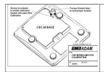
The calibration of the CBC-M scale is accomplished by removing the label at the base of the scale which covers a hole through which the PCB can be accessed. If your scale is not provided with this hole, you need to break the security seals and remove the top cover to gain access to the circuit boards inside. See the figure on the security seal below.
