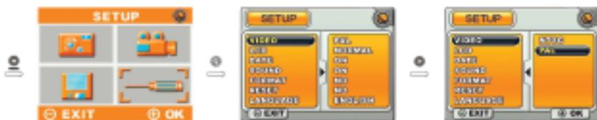
For **VIDEO** playback, select NTSC or PAL. These are the two main television systems used for playback of movies you take. NTSC is used throughout North America as well as in Japan, South Korea, and parts of South America. PAL is used throughout most of Europe, Australia, China, and parts of South America. Using the wrong format will result in blurred or very poor quality movie images.
