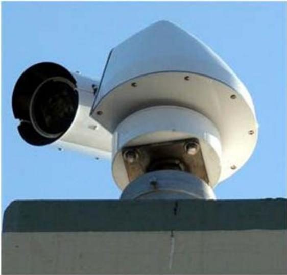
NOTE: The Sidewinder pictured above has been attached to a post-top mount and a custom parapet pole mount.
