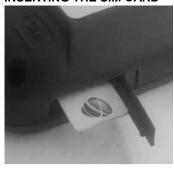
1. Slide the micro-SIM card to the holder from the hole on the side of the unit contacts in the SIM are facing towards keypad and the cut corner of the card inward. Make sure the card locks to holder. Do not use force, as the SIM will go to its place easily.
