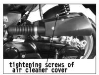
A: Remove 6 tightening screws of air cleaner cover.
