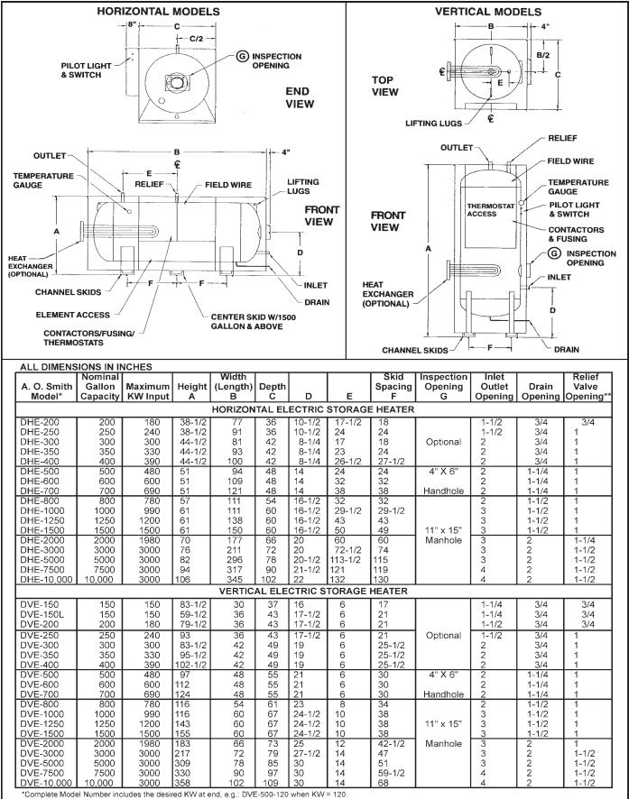
\*Size may vary according to KW input. Minimum installation clearances required: 30" from front, 12" from top, and 24" from right side.
