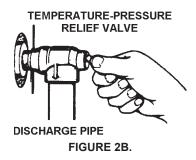
If after manually operating the valve, it fails to completely reset and continues to release water, immediately close the cold water inlet to the water heater, follow the draining instructions in the Operation section of this manual, and replace the temperature-pressure relief valve with a properly rated/sized new one, see Page 9.
