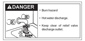
The **TEMPERATURE-PRESSURE RELIEF VALVE** must be manually operated at least once a month. Lift the lever at the top of valve several times until the valve seats properly and operates freely, see Figure 2B.
