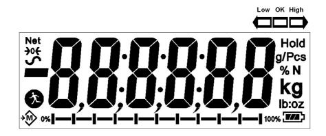
Other symbols will show when a weight has been tared (NET), the scale is at zero and stable, if a value has been stored in memory, or when the animal weighing function has been enabled. A battery symbol will show the state of charge of the internal battery.
