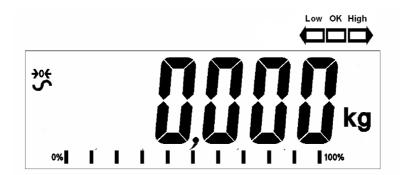
Place a container on the platform and a value for its weight will be displayed.  Press the [0/T] key to tare the scale. The weight is deducted and stored as the tare value leaving zero on the display. The "NET" indicator will be ON and as a product is added only the net weight of the product will be shown. The scale could be tared a second time if another type of product was to be added to the first one. Again only the weight that is added after taring will be displayed.
