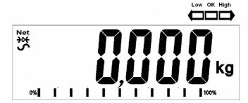
NOTE: The "NET" indicator will only be ON when the tare weight exceeds 4% (+/- 2weighing divisions) of the scale capacity.
