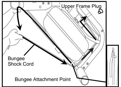
First, move the Rowing Handle to it's farthest forward point on the Mainframe, then cut the plastic end tie and follow the drawing above for bungee removal. Next, remove the Upper Frame Plug to allow the Bungee Shock Cord to be threaded through the top of the frame. Note: You will need to rotate the Belt/Bungee Pulley to align the holes properly. Should the belt drop off of during the bungee change, please refer to the previous pages for "Attaching/Reattaching the Rower Belt".
