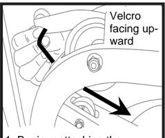
1. Begin reattaching the Rower Belt by threading around the Rower Belt Pulley with the Velcro side facing upward as illustrated.
