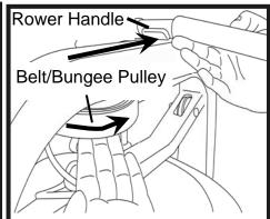
3. Wind the Rower Belt onto the Belt/Bungee Pulley until the Rower Handle is as it's furthest forward position.
