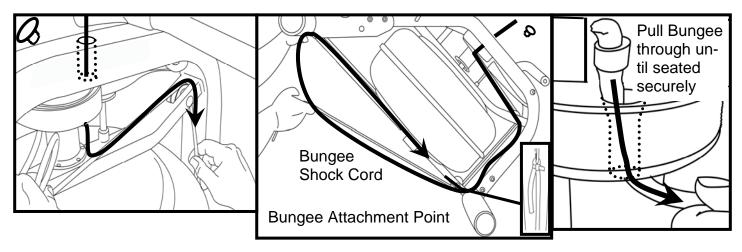
Reinstall the Shock Cord through the Upper Frame, along the opposite side of Idle Wheel, through the Mid Frame and Lower Bungee Pulleys and then tie off with plastic tie wrap to correct tension. Replace Frame Plug.
