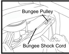
4. Rethread the Bungee Shock Cord (on opposite side of the Idle Wheel) back through the Bungee Pulleys and tie off at the Attachment Point.
