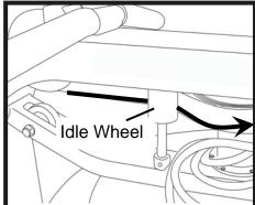
2. Next, thread the Belt around the Idle Wheel as shown.
