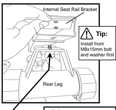
Mount Rear Leg as shown, aligning the M8x15 bolts and washers up through the Rear Leg, the bottom of the Seat Rail and threading into the Internal Seat Rail Bracket as illustrated.
