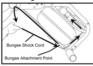
1. To detach belt, simply pull beyond the range of the normal rowing stroke until the belt detaches from the Belt Bungee Pulley.
