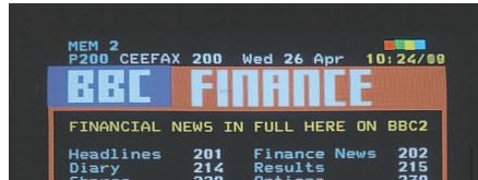
A Teletext page with the colour bar at the top right indicating that it is a Fastext page.
