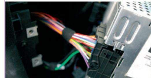
Remove the optical cable and the Quadlock connector. Follow the recommended installation on **Fig 2**. (previous page), connect our Quadlock cable to the Head Unit and connect the original female Quadlock to the male end of our cable. For further details, please check **Fig. 3**.
