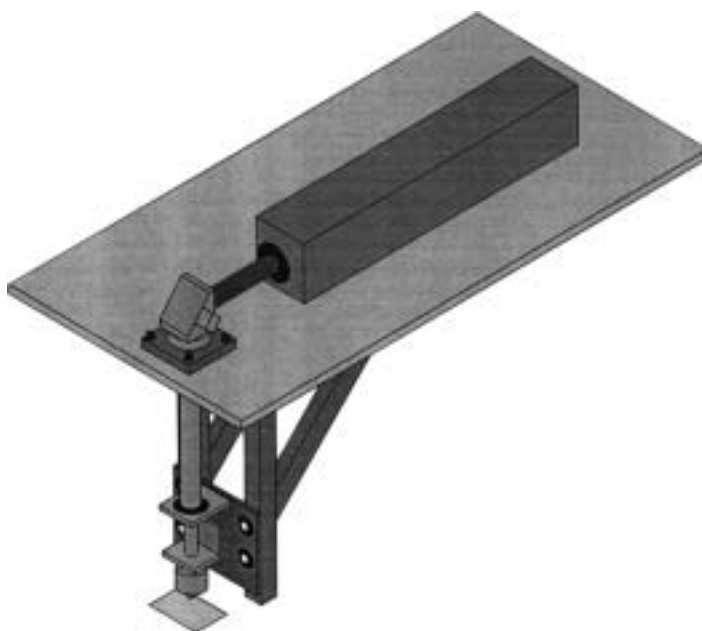
Figure 6. Fixed Laser with Fixed Beam Delivery System
