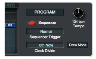
This area to the right is the master section for all four sequencers. Click on the red **LED** to turn the sequencer on and off, adjust **Tempo**, select **Sequencer Trigger** source and choose the **Clock Divide** option to determine the gate time of each step relative to the tempo.
