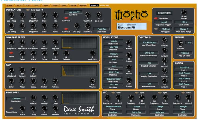
The Mopho PlugSE™ Editor displays a faithful reproduction of the Mopho's front panel. Every knob, switch, and rotary control is exactly as you would find it on the Mopho, and all Editor controls are interactive and functional. Changes made anywhere on this panel will cause corresponding changes to be made on the Mopho hardware, and also sent to the DAW (host) automation while recording.
