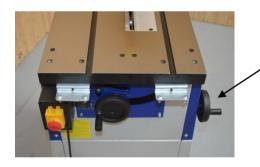
Raise the blade with the hand wheel at the front of the machine. Fit the handwheel from the bag of components to the spindle on the R/H side of the saw, tighten the grubscrew and turn the wheel until the blade is vertical
