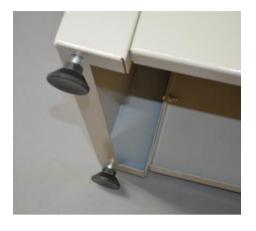
While the machine is on its side, take the four feet from the bag of parts and screw them into the four holes in the base. These feet can be adjusted by means of a spanner so that saw table is level after the machine has been put in place.
