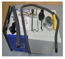
Lay the saw over on its front and remove the two bolts holding it to the pallet. Support the bottom of the saw as you remove the second bold. There is little weight at this end of the saw, so one hand is adequate. Discard the pallet and remove from the interior of the saw base 2 flexible tubes, 3 jubilee clips, the crown guard, the tube support, the reducer and a bag of parts.
