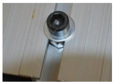
Fit the front travel stop. This is the loose nut and bolt that that was in the cardboard box with the guide rails.
