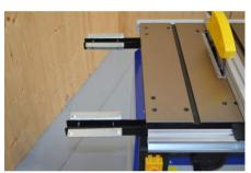
Fit the two brackets which will carry the guide rail for the sliding carriage. These are bolted to the left hand side of the table with the setscrews provided. Leave them slightly loose until the guide rail is in place. Fit the guide rail in a similar way to that with which you attached the front and rear guide rails. Make sure that it is parallel to the saw blade
