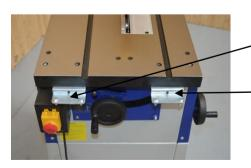
There are two brackets at the front of the saw table and a similar pair at the back. Each one has two hex headed bolts and nuts passing through it and a small black adjuster at the back
