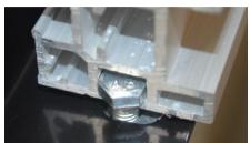
The extrusion with the scale should be fitted to the front of the table, scale uppermost and in both cases the wide groove should face outwards. If they are difficult to slide on, make sure that you have slackened the nuts sufficiently and rock the extrusions gently as you move them along. You may need to reach round to the back of the brackets and unscrew the black adjusters a little, if they are binding on the aluminium.
