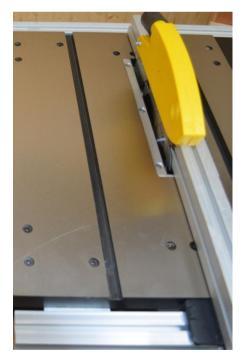
Align the fence with the saw blade and holding it in position, align the 0 on the scale with the left hand edge of the black portion of the fence.
