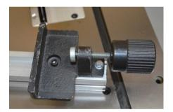
Join the two parts of the rip fence using one cap head setscrew and one hex head bolt.
