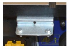
Loosen the nuts and lifting each bolt head in turn, slide one of the two longest aluminium extrusions over them
