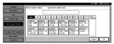
If a destination protection code is set, the entry screen appears. Enter the protection code for destination using the number keys, and then press **[OK]**.
