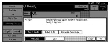
To use ID Override Transmission, select [ID Override Transmission], and then specify a 4-digit ID using the number keys and [A], [B], [C], [D], [E], and [F].
