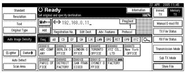
It is not necessary to press [Add] when adding destinations using the destination list.
