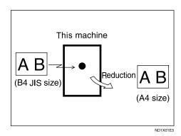
If A4 paper is loaded and a document of B4 JIS size is received, the machine will reduce the document to a single A4 sheet.
