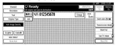
2 After checking the settings on the display, press the [Check Modes] key. The display before the [Check Modes] key was pressed appears.
