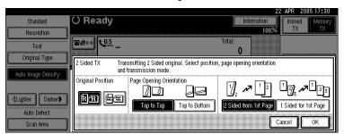
Make sure that the specified original position matches the orientation of originals loaded in the ADF.
