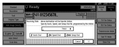
To specify a Receiving Station using the Transfer Station's Speed Dial, select [#X Speed Dial], and then enter the number of the Speed Dial code.
